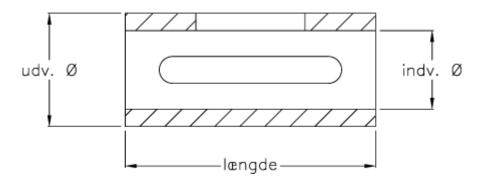
Description = 9/11Internal diameter = 9Length = 22Outer diameter = 11
